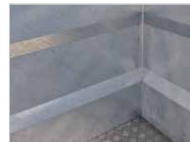
All-welded monocoque construction with aluminium 'tread plate' floor for safety, lighter weight benefits and easy cleaning for bio-security purposes.
