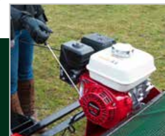
The MSP120 is powered by a Honda 5.5hp engine, with its legendary reliability and easy pull start system. This power unit gives the sweeper complete independence so that it can be towed by any suitable vehicle, depending on the location and conditions.
