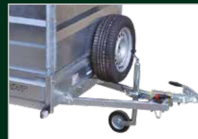
Other options include a spare wheel with WB103 mounting bracket and RT710-01 jockey wheel.
