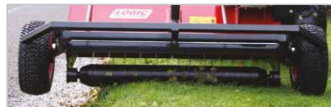
The full width anti-scalping roller (above) protects the sward from scalping and allows cutting over kerbs.
