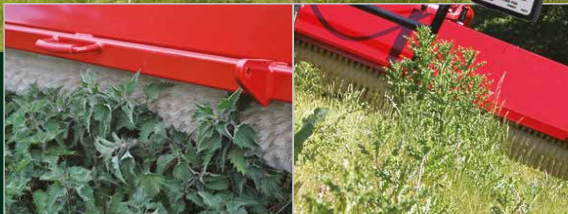
Seen here treating nettles and thistles saving valuable clover and grass. The brush section build up allows treatment on slopes (above right) without the danger of run-off, common in some carpet type systems.
