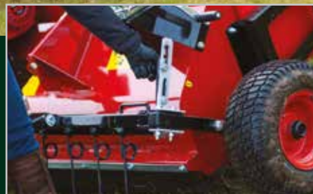
The optional MSP121 tine bar is easily fitted and adjusted to contact more solid heaps of rubbish or animal droppings, breaking them up before the brush. It is easily adjusted by turning the large hand screw (above) to release and reposition the bar stem into one of 3 secure locating slots.
