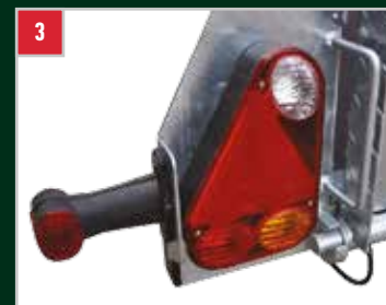
3 Protected light cluster with inbuilt triangle, lenses and marker lights.
