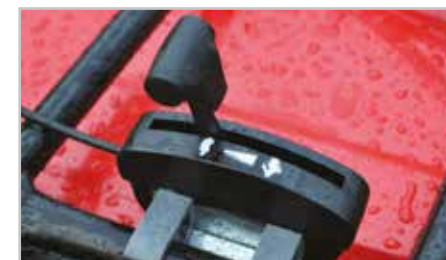
Throttle control is positioned close to hand and allows instant build up from idle, when required. Brush engagement is controlled via a centrifugal clutch which starts the brush when the engine revs are increased.
