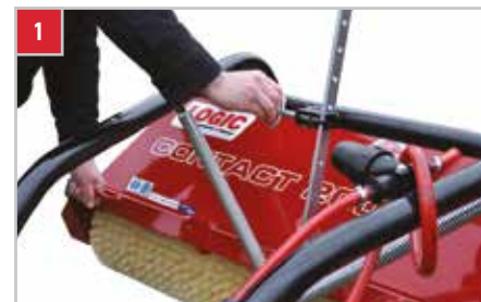
Height adjustment is spring-assisted to allow the machine to be quickly and easily set to the correct working height for the weed infestation being treated.
