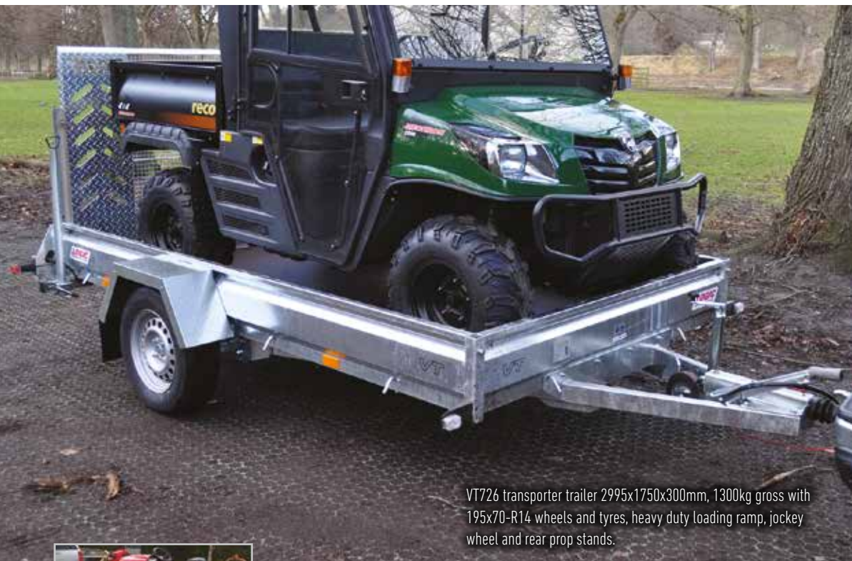
1 Prop stands to support the trailer when loading vehicles.
