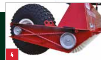
The contra-rotating brush is ground driven from the wheel using a segmented 'V' belt housed under a robust, protective cover. Low ground pressure tyres on bead-lock rims allow for use in soft, wet ground and provide suspension for the unit when working in rough conditions.
