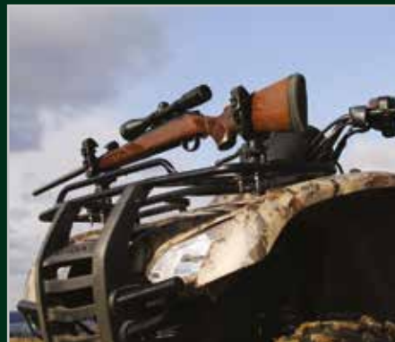
KOL21510 Rhino XL grips (left) on the front carrier of this ATV for secure rifle mounting which allows quick access.
