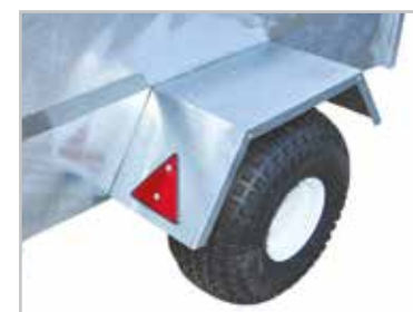
Optional - MGXXX mudguard kit to protect animals and operator from flying mud. Various sizes to suit wheel options.
