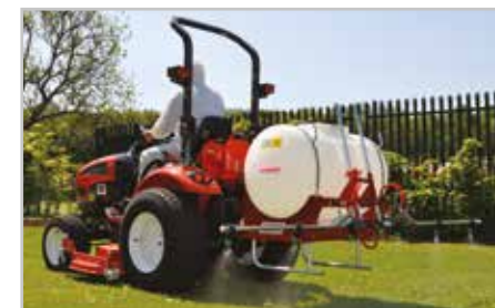
Perfect for small tractors with 'Cat 1' linkages like this compact tractor mower unit. The skid unit sets the sprayer at a good height for dismantling and storage.
