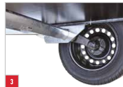
Standard Al-Ko axle with progressive rubber suspension giving an excellent smooth, quiet ride.
