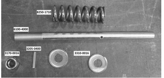
Assemble the pivot as shown below. Apply grease between the cup and round tube to ensure smooth operation. Use a pair of pliers to hold the roll pin when doing up the nyloc nut with a spanner.
