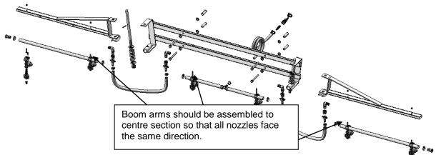
The following parts are required to attach each boom arm to the centre section
